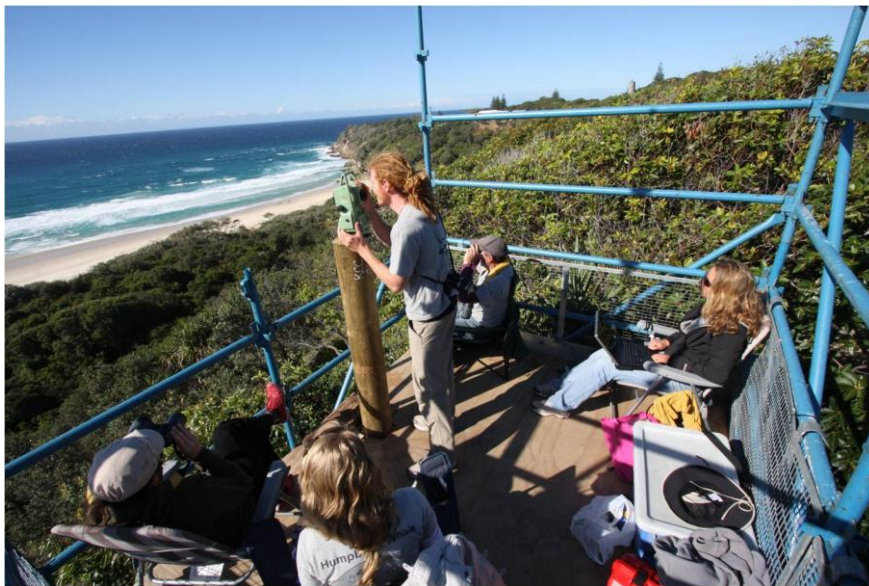
Figure 5. The modified tower was an excellent survey platform. Although the platform itself moved slightly and vibrated, the theodolite was mounted on the top of a thick pole which went through the platform floor to the ground and which was securely fixed to the underlying wooden platform. This provided great stability. In this photo we can see the theodolite operator (standing), the computer operator (right) and the three spotters looking at their respective sectors (from left to right: south-east, east and north-east).
